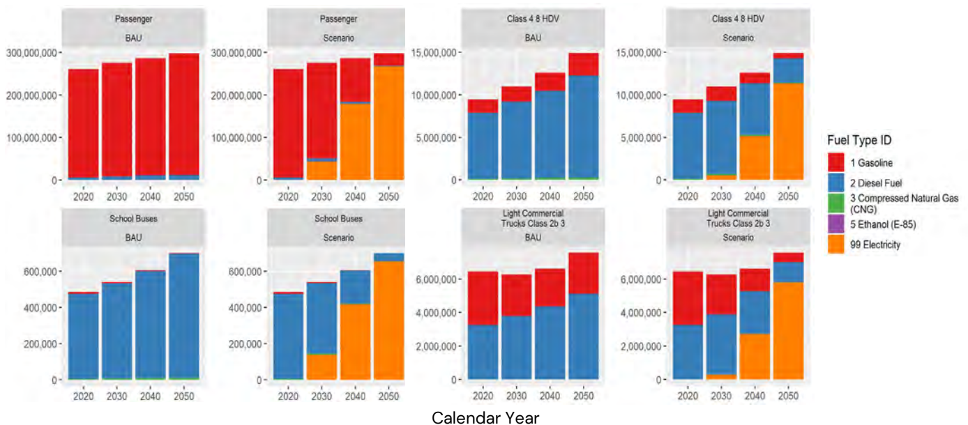
Figure ES-1. Modeled vehicle populations in the four vehicle categories and five fuel types under the BAU and vehicle electrification Scenario
